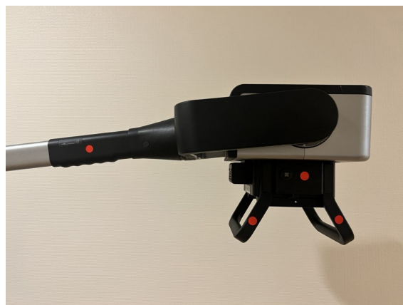
Figure 2. Landmarks (red circles) for touch on the X-ray tube. These landmarks served not only to limit the spread of the virus but also to economize time and labor to sanitize the X-ray tube.
